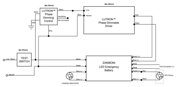
(1) DO NOT CONNECT UNTIL INSTALLATION IS COMPLETE AND AC POWER IS SUPPLIED
